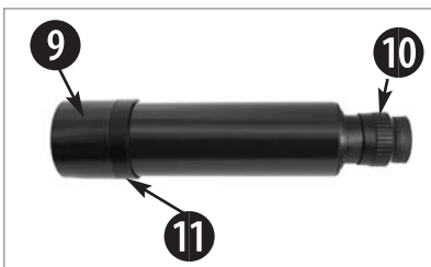
Fig. 40c: 8x50 Viewfinder tube: Objective lens (7), eyepiece/focuser (8) and locking ring (9).
