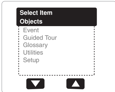
Fig. 44a: The menu displays on the top line and Menu options display on the second line. Use the Scroll keys to move up or down through the list of options. Press ENTER to select the desired option.
