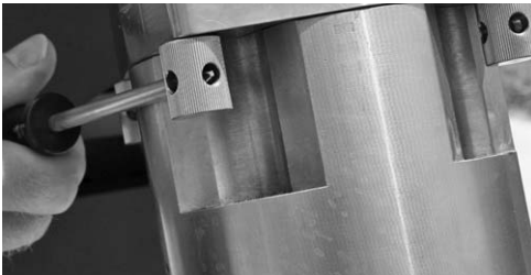
close up of indentation on fixed counterweights
