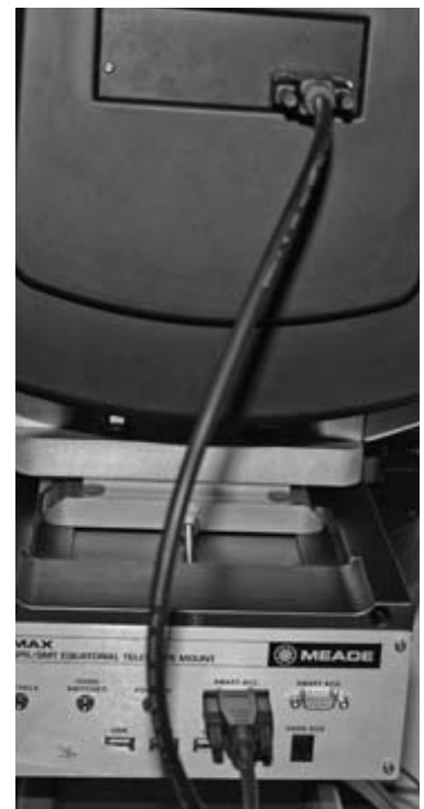
JUMPER CABLE BETWEEN OTA AND SADDLE PANEL (may use either of the Smart Accessory ports)
