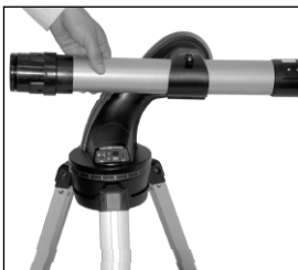
Fig. 7: Attach and balance the optical tube.
