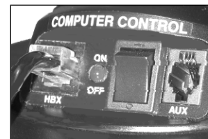
Fig. 12: Connect Autostar to the HBX port.
