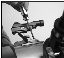
Fig. 8b: Attach the viewfinder bracket to the reflector optical tube assembly.
