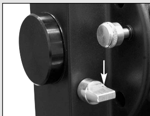
Fig. 29b: Flip mirror control in the “down” position.
