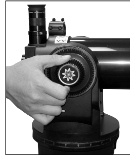
Fig. 16: Tighten vertical lock.
