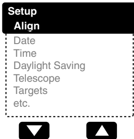
Fig. 26: Menu options display on the second line. Use the Scroll keys to move up or down through the list of options. Press ENTER to select the desired option.
