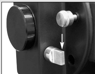
Fig. 29a: Flip mirror control in the “up” position.
