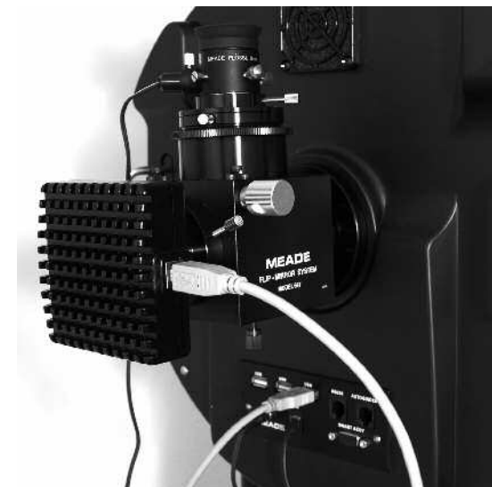
Fig. 38b: The Deep Sky Imager connected to the RCX400 with a flip mirror optional accessory.
