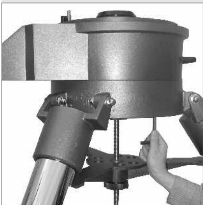
Fig. 62: Attach the drive base to the tripod.
