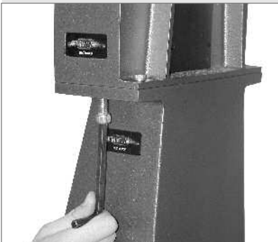
Fig. 67: Tighten the fork arm assembly using the provided hex key.
