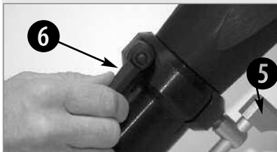
Fig. 10: Tighten the leg adjustment lock (6).
