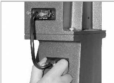
Fig. 68: Plug in the DB-9 and DB-25 connectors to provide power from the Dec. motor to the fork arms.
