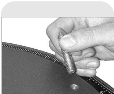
Fig. 61: Remove the pointed bolts from the drive base.
