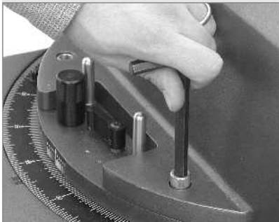
Fig. 63 Bolt the fork to the drive base.
