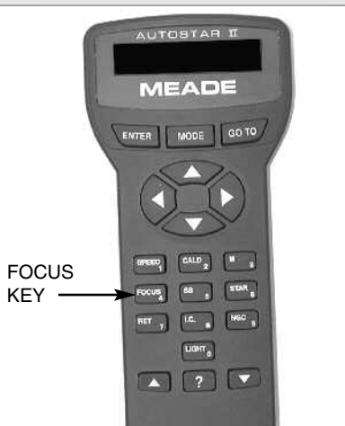
Fig. 25: Focus is all-digital, using the Focus key (the #4 Number key) of the AutoStar II handbook.
