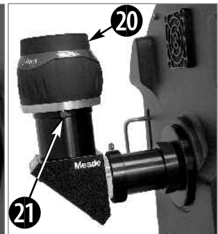
Fig. 20: Slide eyepiece (20) into the diagonal mirror and tighten thumbscrew (21).
