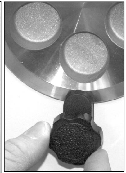
Fig. 18: Tighten the tension adjustment bolt as necessary.
