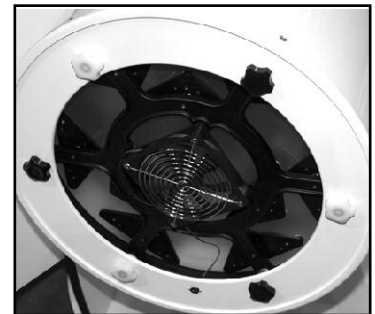
Fig. E: Some models come with knobs instead of screws. Use the black knobs to adjust collimation and the white knobs to lock collimation.
